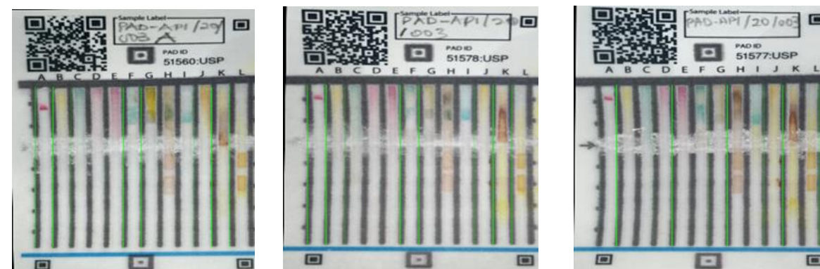
Figure 2c: Results of a falsified azithromycin formulation
