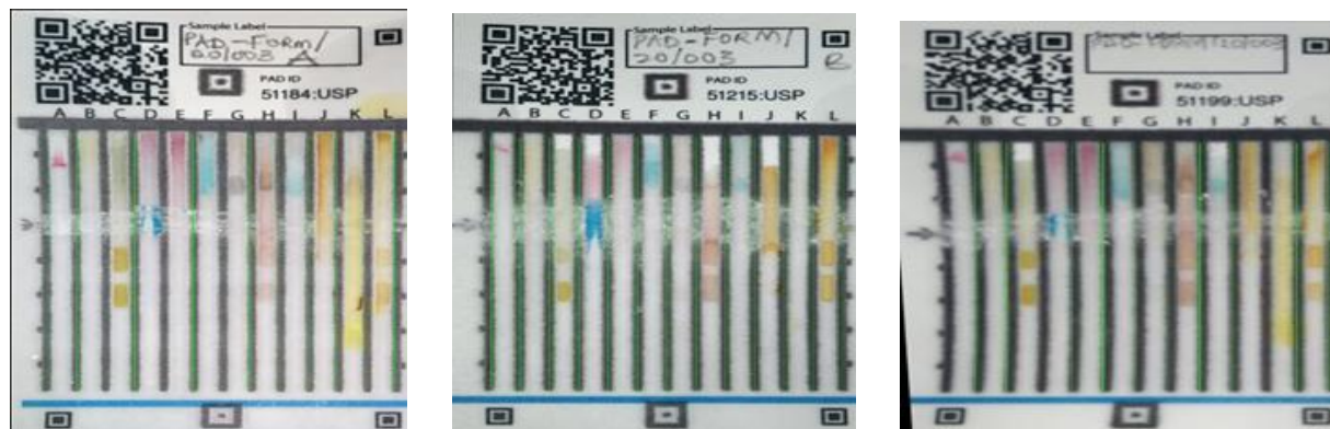
Figure 5b: Results of a substandard ciprofloxacin formulation
