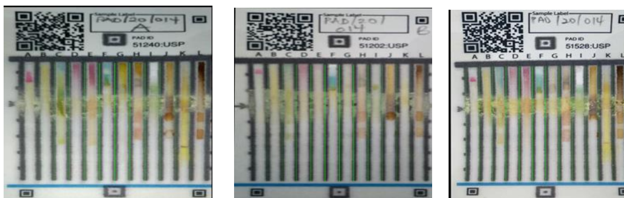
Samples containing the correct amount of doxycycline showing the correct color on lane L (brown).
