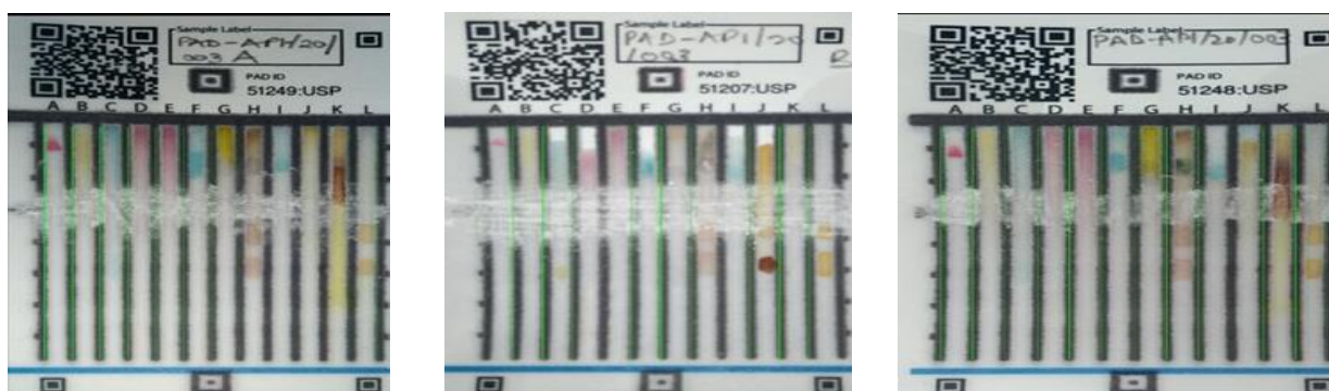
Figure 4c: Results of a falsified chloroquine formulation
