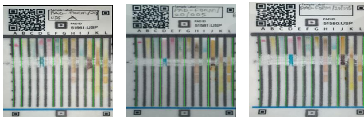
Figure 2b: Results of a substandard azithromycin formulation
