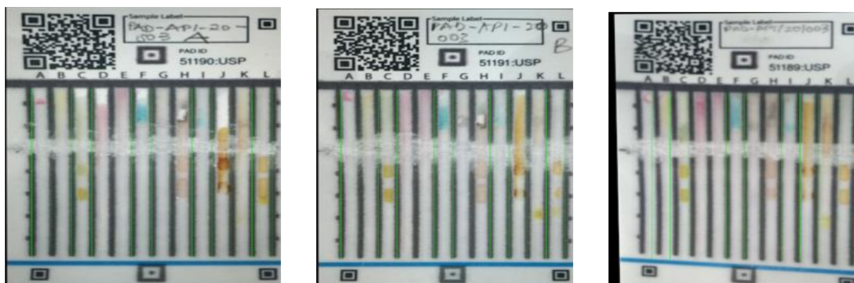
Falsified formulation of ciprofloxacin showing different colors on lanes D and L
