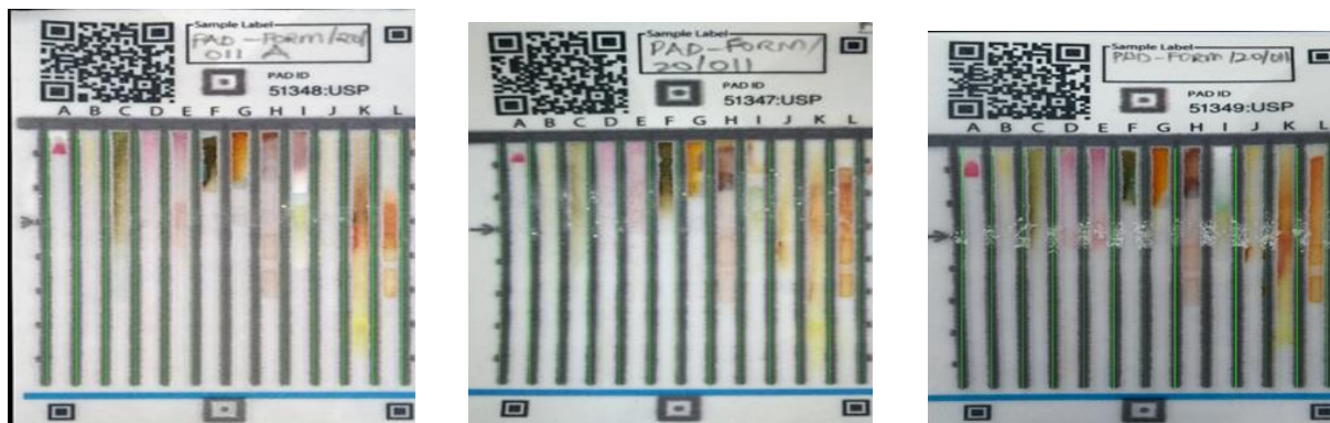
Figure 3b: Results of a substandard ceftriaxone formulation
